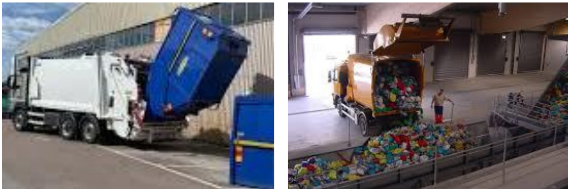
Figure 31. Large tipping containers being emptied (l) and mixed collection of different-colored bags 63
