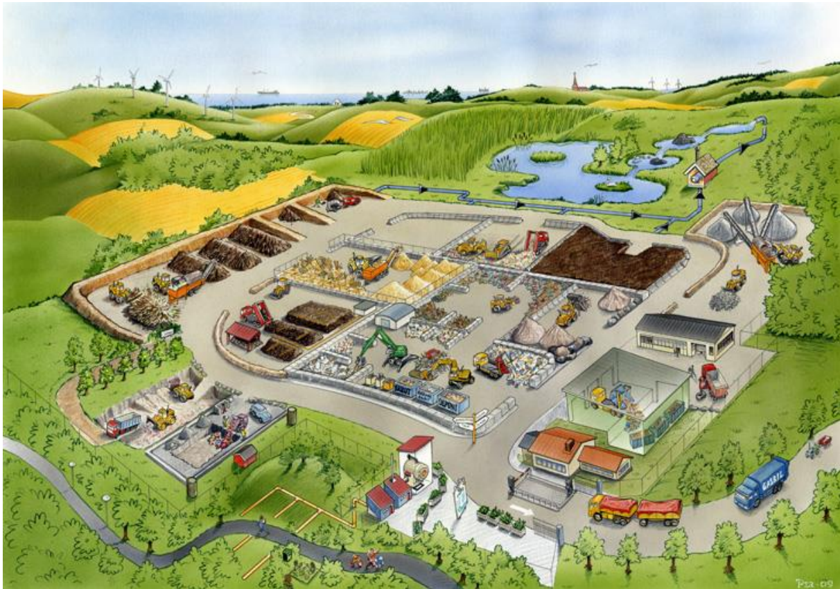
Figure 45. Example of a waste treatment facility including a sanitary landfill, windrow composting, wood chipping, gravel production etc.
